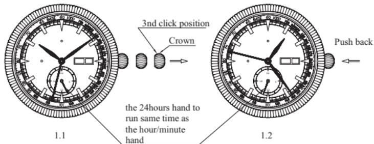
**Imporant notice :** 1. Push-buttons must not be used during the period of 9pm (evening) till 3am (morning), as otherwise the movt will be damaged.
